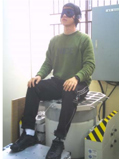
Fig. 5. Vibration shaker and posture of subject. (upright, footrest and the palms slightly resting on the knees)
